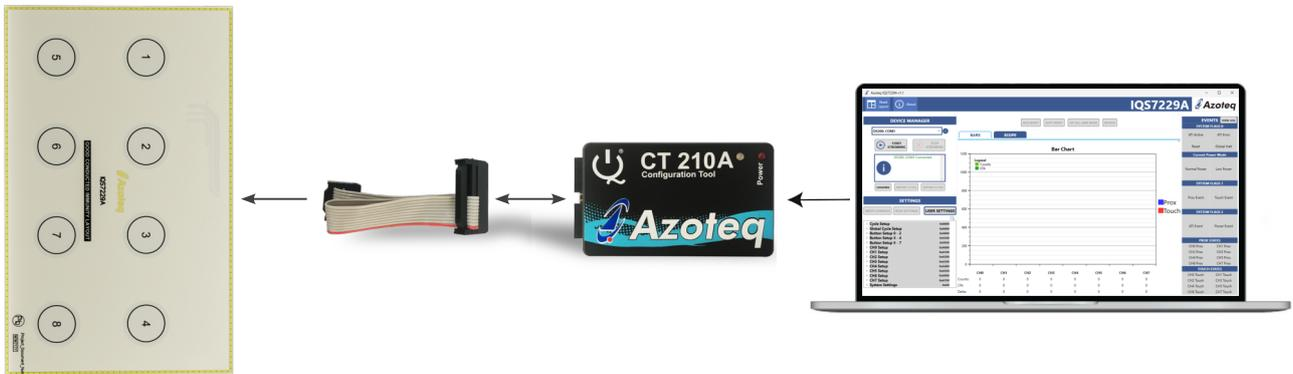
Figure 2.3: CT210A Connection for Streaming and Testing
