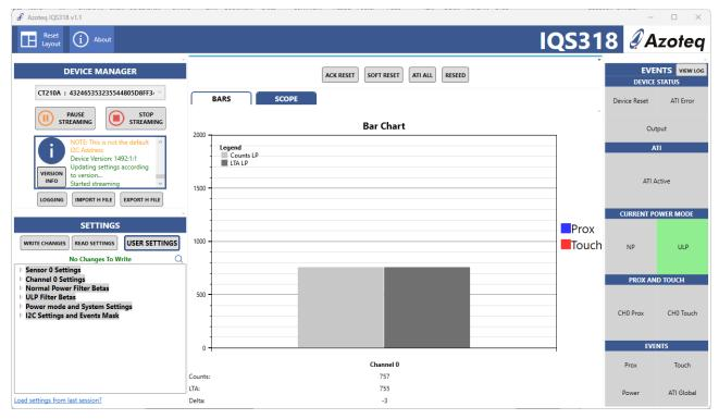
Channel 0 represents the Inductive Key. This triggers in a downwards directions, meaning a push down on the key will result in a decrease of the counts.
