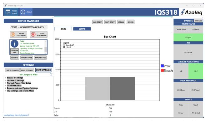
Channel 0 represents the Self Capacitance Switch. This triggers in both directions, meaning if the hinge is opened to lie on top of the electrode the counts will increase and when removed from the electrode the counts will decrease.
