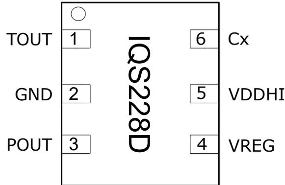
Figure 2.1: DFN-6 Pin-out
