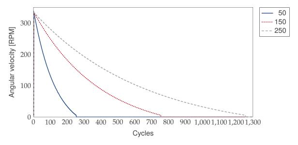
Figure 8.3: Freewheeling Response as Inertia Changes
