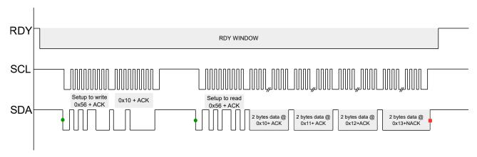
Figure 9.1: Example of Reading Data over I<sup>2</sup>C
