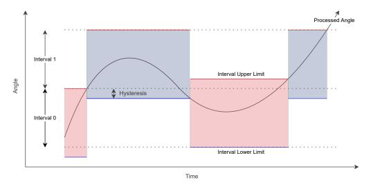
Figure 5.2: Illustration of the Interval Size and Interval Hysteresis
