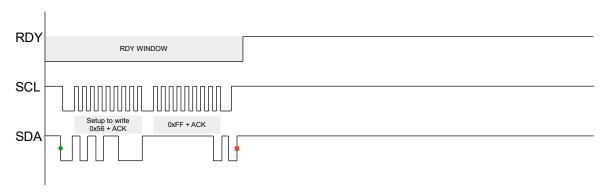
Figure 9.2: Force Stop Communication Sequence
