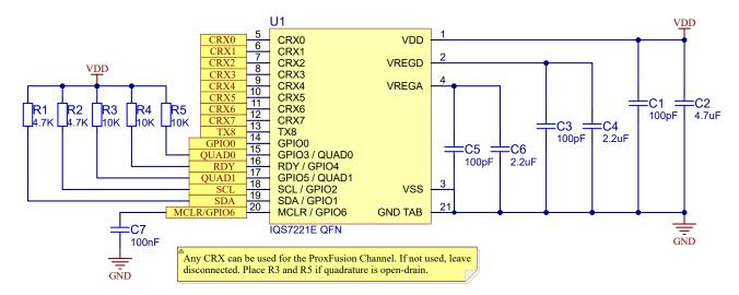
Figure 2.1: IQS7221E QFN Reference Schematic
