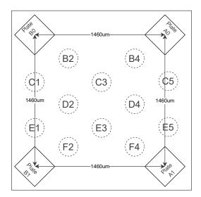
Figure 2.4: Plate Layout WLCSP (Top View)
