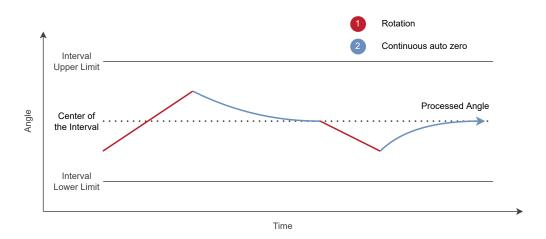
Figure 5.5: Continuous Auto-zero Behaviour
