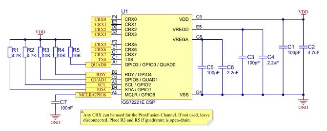
Figure 2.2: IQS7221E CSP Reference Schematic
