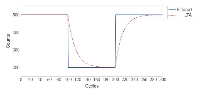
Figure 6.1: Channel Filtered Counts and LTA Response during a Touch Event, with the Release UI Enabled
