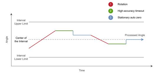
Figure 5.4: Stationary Auto-zero Behaviour
