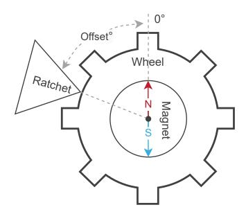
Figure 5.3: Illustration of the Absolute Angle Offset
