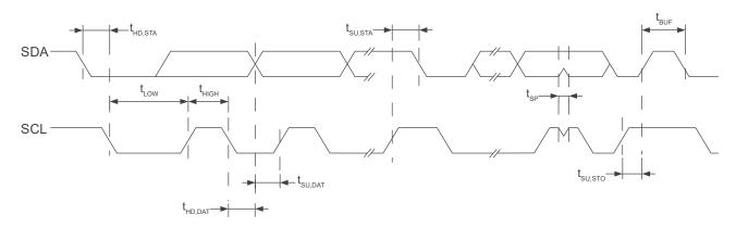
Figure 4.2: I<sup>2</sup>C Mode Timing Diagram
