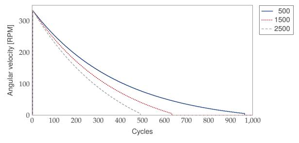
Figure 8.1: Freewheel Response as Friction Changes
