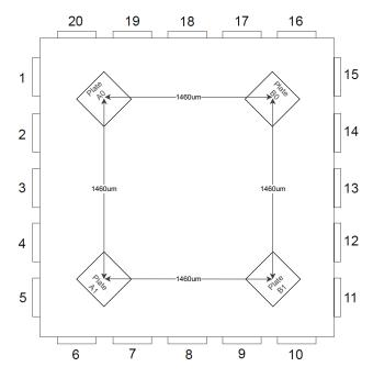
Figure 2.3: Plate Layout QFN (Top View)
