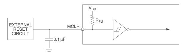
Figure 4.1: MCLR Pin Diagram
