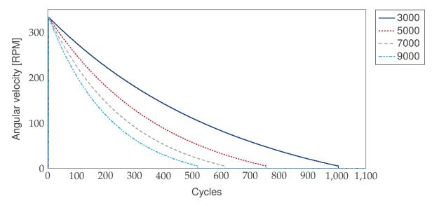
Figure 8.2: Freewheel Response as Damping Changes
