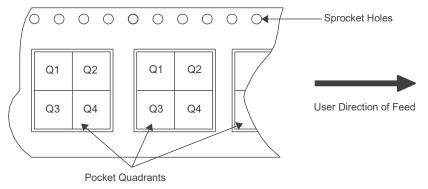
Figure 12.4: Tape and Reel Specification
